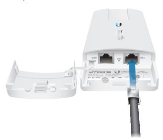
3. Connect the other end of the cable from the *DATA* port to the Ethernet port labeled **POE** on the *airFiber PoE Adapter*.
