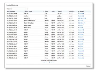
It reports the MAC Address, Device Name, Mode, SSID, Product type, Firmware version, and IP Address for each Ubiquiti device. To access a device configuration through its web management interface, click the device's IP address.
