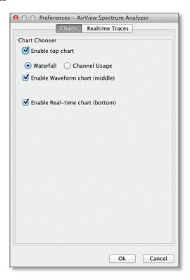
**Enable top chart** Check the box to enable the top chart. Select the desired chart to display in the top chart panel on the main view. There are two options:
