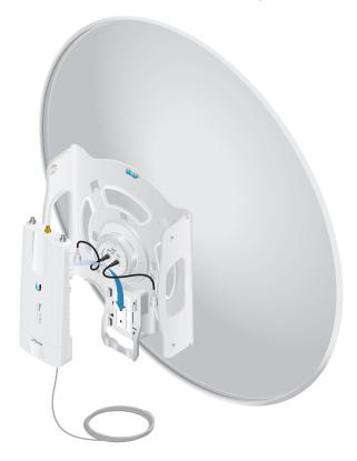
2. Attach the RF cables from the antenna feed to the RF connectors on the AF-5X in this combination: +45° to Chain 0 and -45° to Chain 1.
