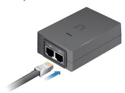
4. Connect the *Power Cord* to the power port on the *airFiber PoE Adapter*. Connect the other end of the *Power Cord* to a power source.
