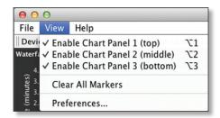
**Enable Chart Panel 1 (top)** Displays the Waterfall or Channel Usage chart in Chart Panel 1, depending on which option you have selected in *Preferences*. This time-based graph shows the aggregate energy collected or channel usage for each frequency since the start of the airView session.
