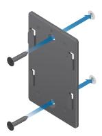
3. Attach the *airFiber PoE Adapter* to the bracket by aligning the four slots and tabs, and then slide the adapter downward.
