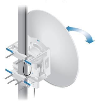
b. Loosen the six elevation bolts, and use the hex nut on the elevation rod to adjust the elevation.
